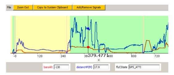
Here, the value tracker is currently at time 379.477, baroAlt has the value -130, and distanceHp has the value 17.9. The state signal flyCState has the value GPS\_ATTI.
